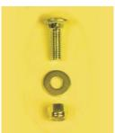
IMPORTANT: TIGHTEN THE NUT TO SEAT THE HEAD OF THE BOLT THEN LOOSEN THE NUT 3/4 TURN. THIS WILL ALLOW THE LINER TO EXPAND AND CONTRACT WITH TEMPERATURE CHANGE.
