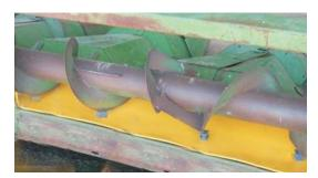
7. Press the Poly panel against the metal by inserting the wooden shims blocks at each auger flight as illustrated below. Snap into place. A putty-knife can also facilitate this process, if needed.
